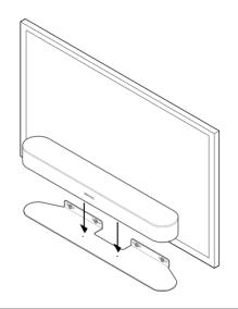
Insert and tighten Beam to the bracket using the mounting screws.
