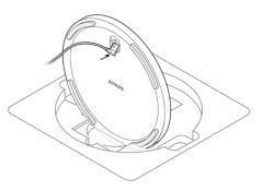
Position the washer with the alignment pins facing in. Then align the stand pole with the base, using the alignment pins to guide you.
